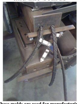
These molds are used for manufacturing waste reinforced steel-belted tires and waste thermoplastic.
