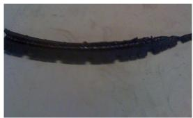
Small piece of steel-belted tire which can be used as a reinforcement element for; asphalt potholes, concrete, adobe, or cement blocks
